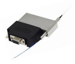
Based on a proprietary thin film cavity filter technology, Agiltron offers Fiber Optic Tunable Filters with central wavelengths of 1060nm, 1310nm, 1550nm and 2000nm. It is tunable continuously over a wide spectral range up to 80 nm. The wavelength tuning is actuated by driving a build-in precise stepper motor through interface of USB or RS232.
